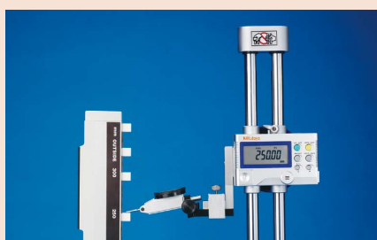
Checking accuracy of height gage
